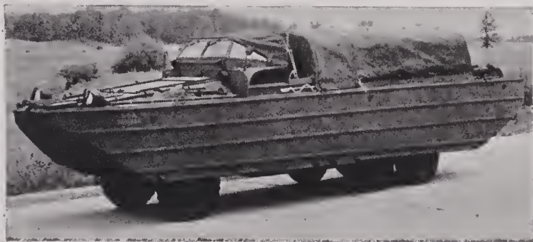
FIGURE 25. Late 1944 production model of 2½-ton, 6x6 DUKW.
